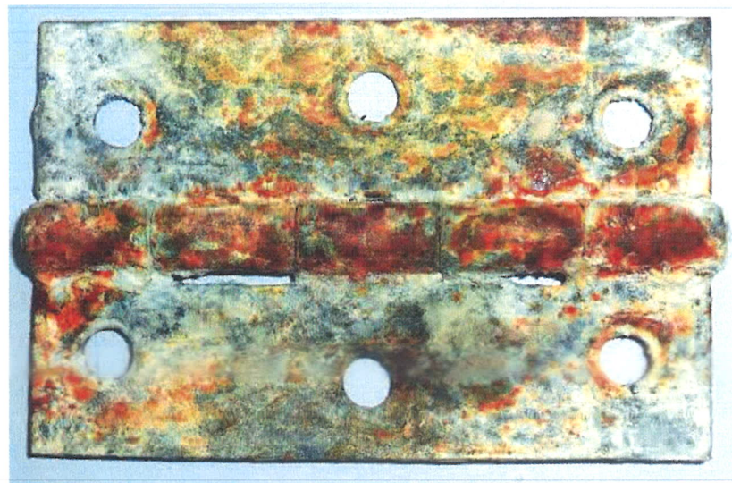
Photograph of Butt hinge after 840 hours
